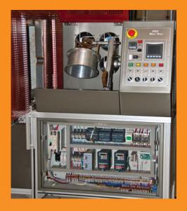
The mini-shuttle rotational molding machine BSE-400 has been designed to make prototypes or for resins quality control purposes. Small-size products with specific wall thickness or products with small production runs are ideal with this machine. BSE-400 is engineered specifically as a tool to invent products.
